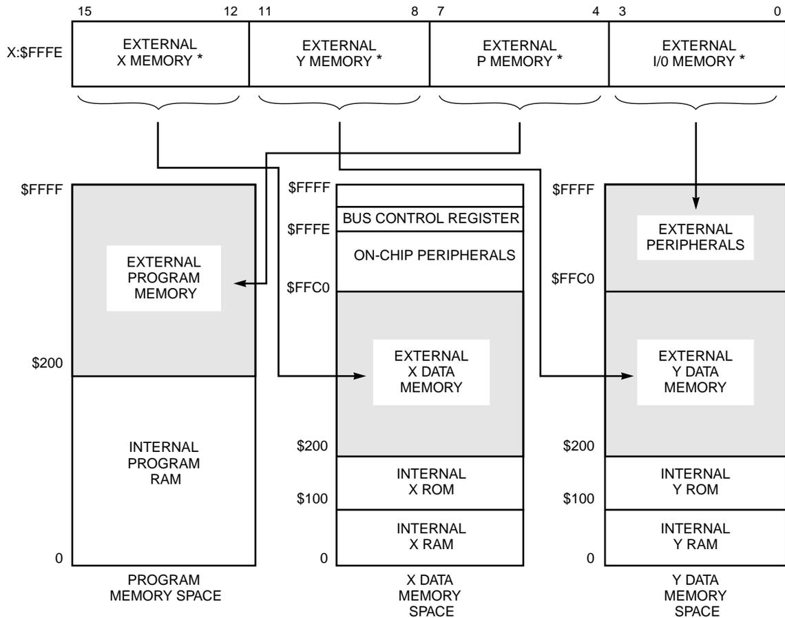
\* Zero to 15 wait states can be inserted into each external memory access.
