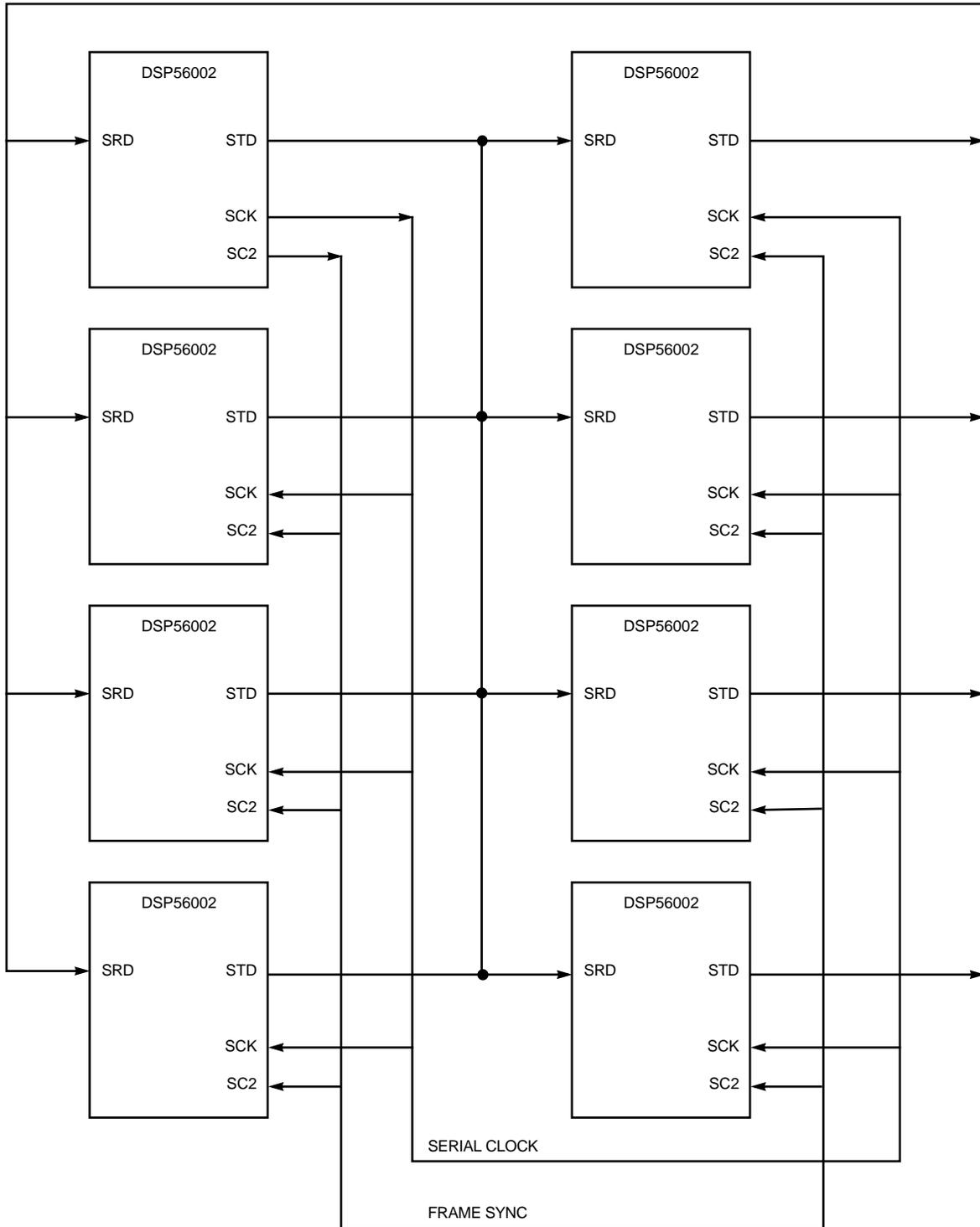
Figure 6-93 SSI TDM Connected Parallel Processing Array
