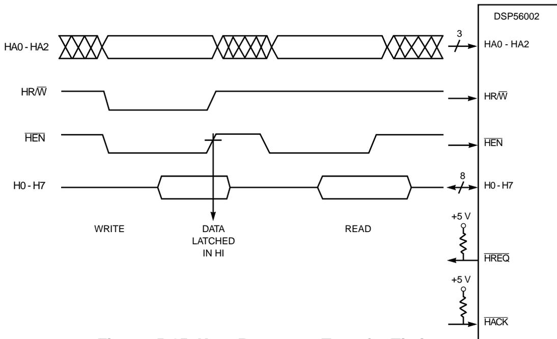
**Figure 5-15 Host Processor Transfer Timing**
