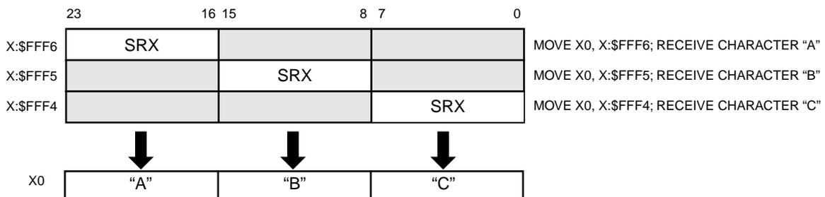
NOTE: SRX is the same register decoded at three different addresses.
