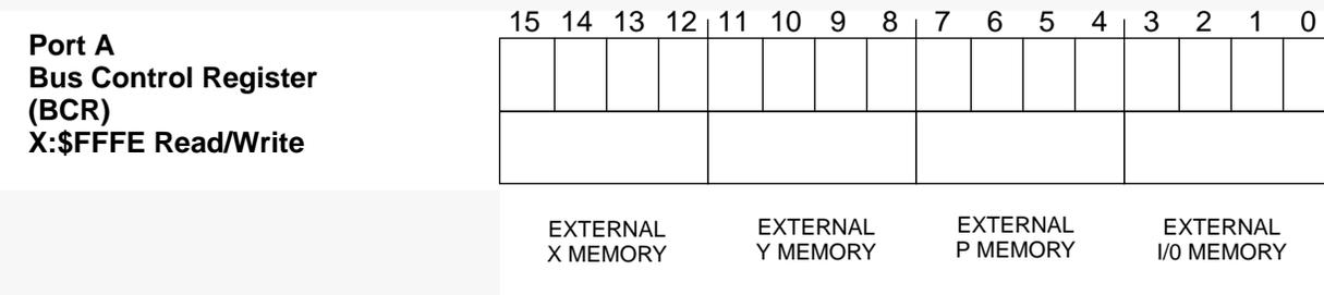
**Figure B-3 Bus Control Register (BCR)**
