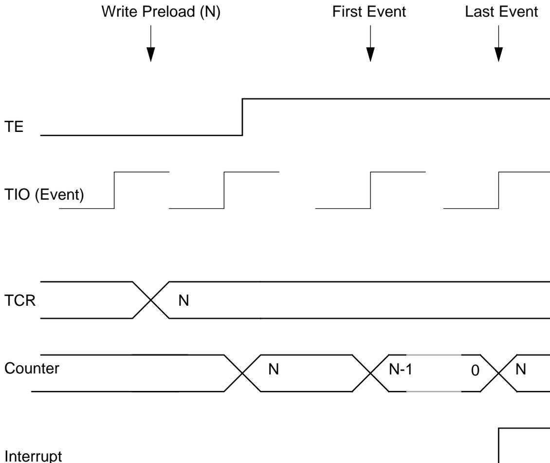
Figure 7-14 Standard Timer Mode, External Clock (INV=0)
