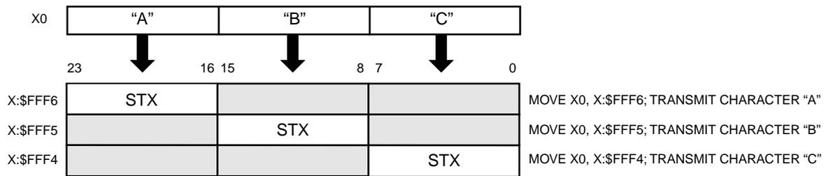
NOTE: STX is the same register decoded at three different addresses.
