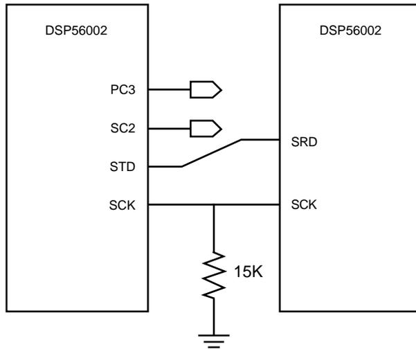
Figure 6-84 On-Demand Mode Example — Hardware Configuration
