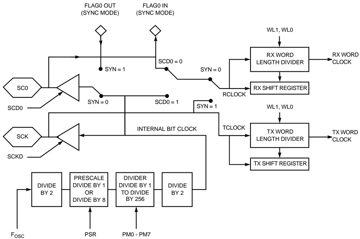
Figure 6-42 SSI Clock Generator Functional Block Diagram
