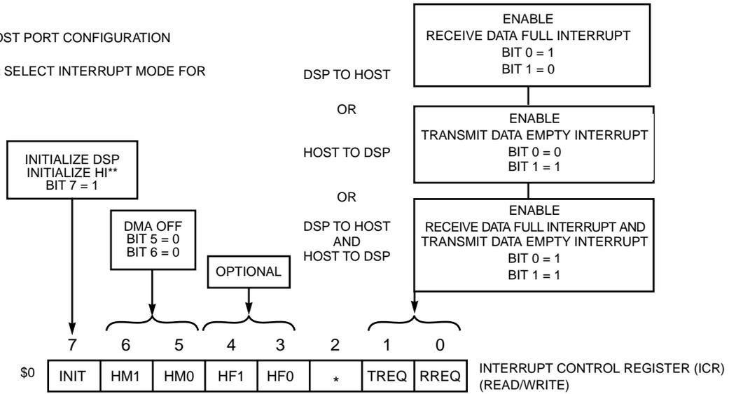
**2. OPTION 4: LOAD HOST INTERRUPT VECTOR IF USING THE INTERRUPT MODE AND THE HOST PROCESSOR REQUIRES AN INTERRUPT VECTOR.**
