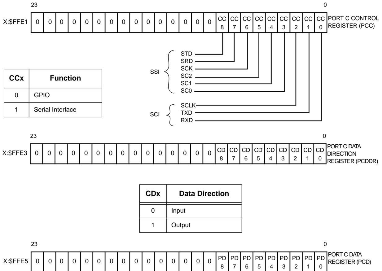
NOTE: Hardware and software reset clears PCC and PCDDR.
