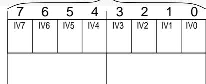
**Figure B-21 Interrupt Vector Register (IVR)**
