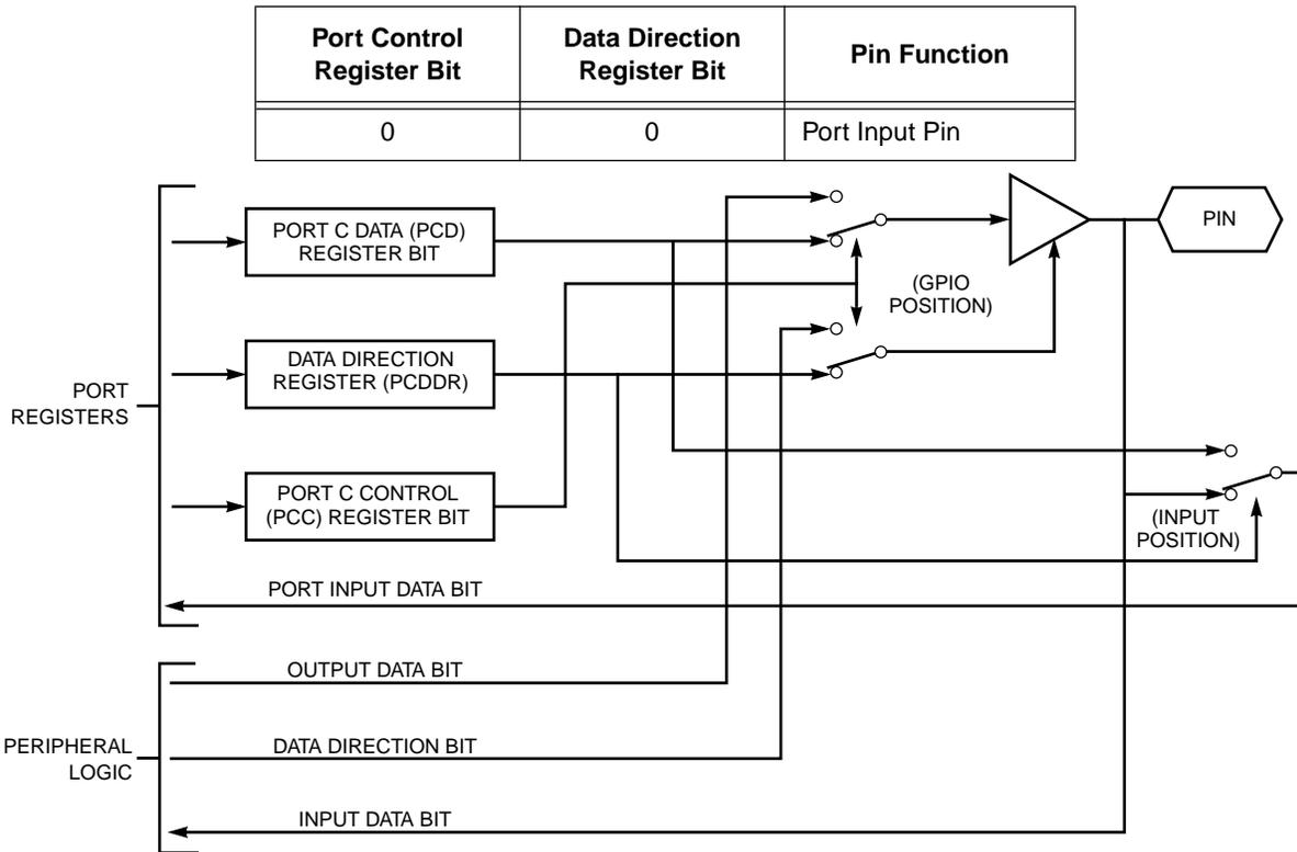
Figure 6-4 Port C I/O Pin Control Logic
