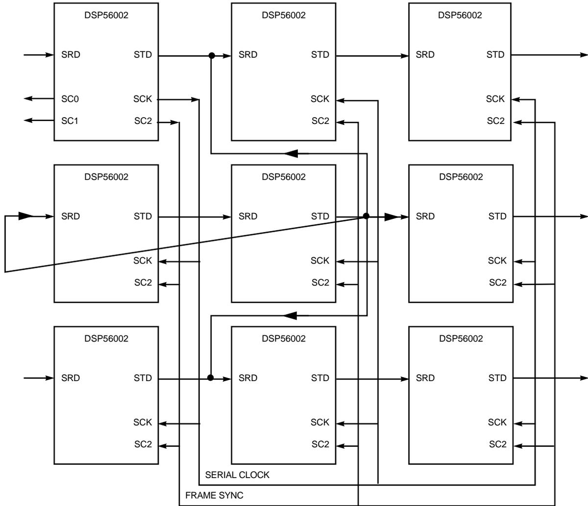
Figure 6-95 SSI Parallel Processing — Nearest Neighbor Array
