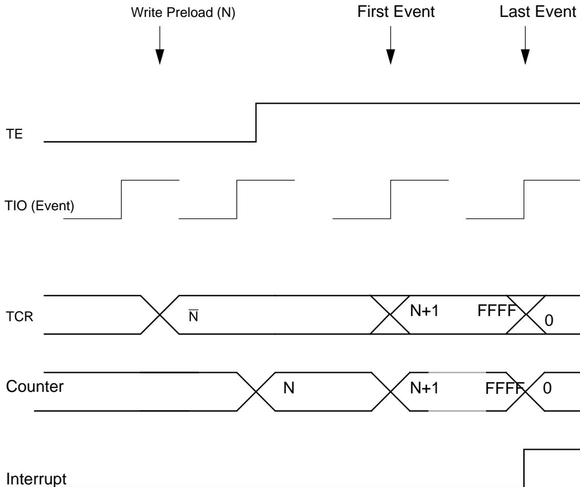
Figure 7-12 Standard Time Counter Mode, External Clock (INV=0)
