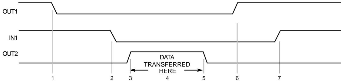
Figure 4-13 Two DSPs with External Bus Arbitration Timing
