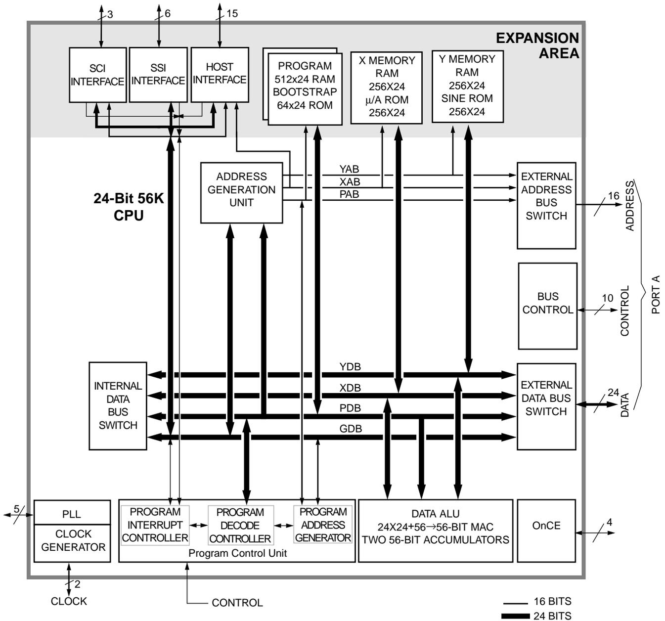
Figure 1-2 DSP56002 Block Diagram
