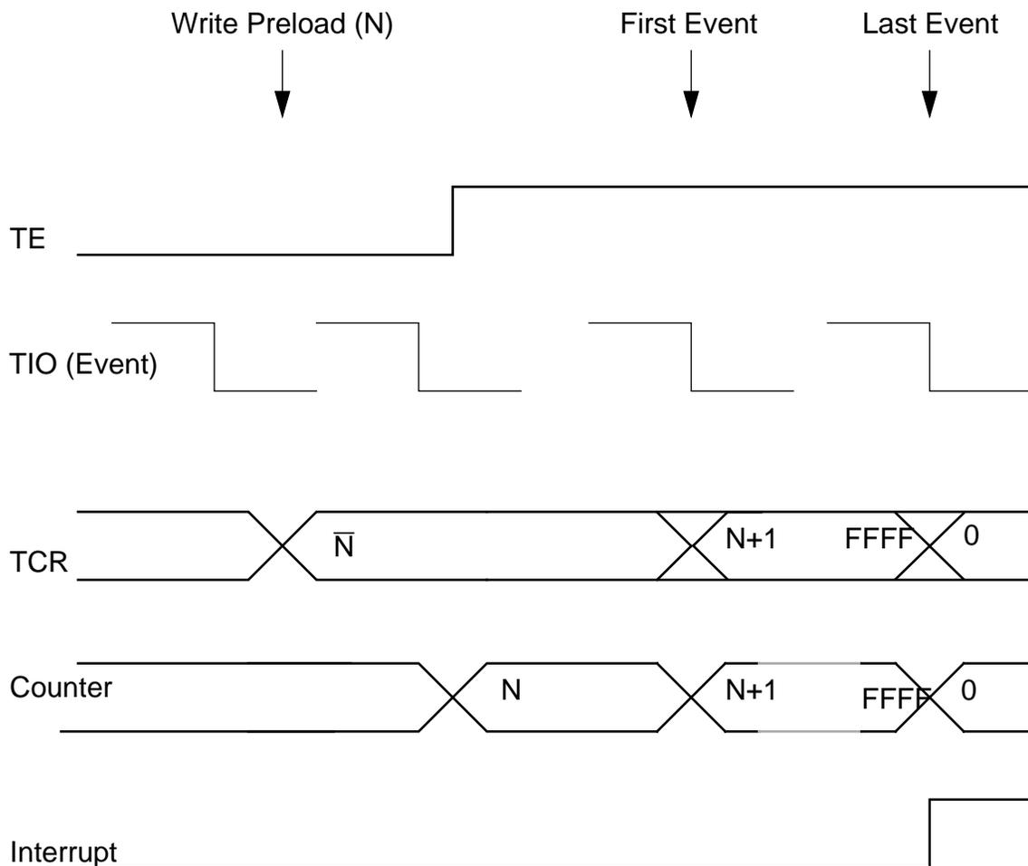
Figure 7-13 Standard Timer Mode, External Clock (INV=1)
