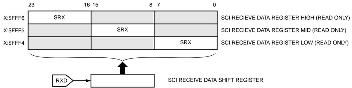
NOTE: SRX is the same register decoded at three different addresses.
