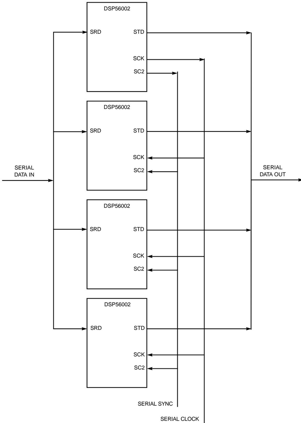
Figure 6-92 SSI TDM Parallel DSP Network
