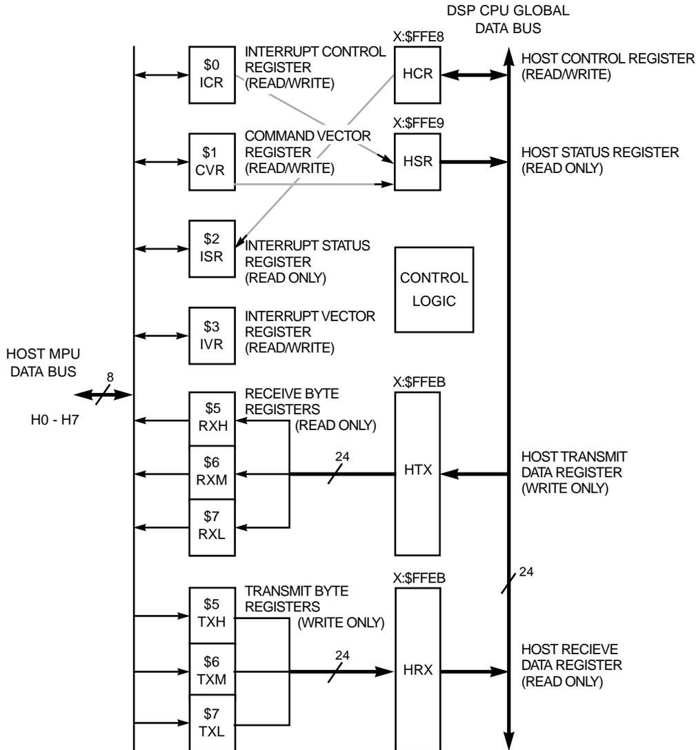
**Figure 5-8 HI Block Diagram**
