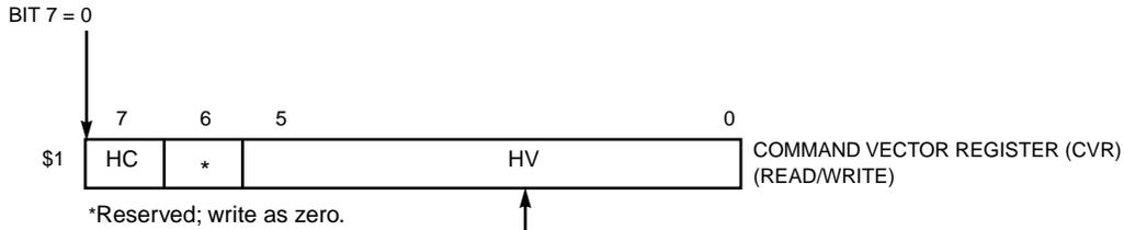
2. **OPTION 1: SELECT HOST VECTOR (HV)** (OPTIONAL SINCE HV CAN BE SET ANY TIME BEFORE THE HOST COMMAND IS EXECUTED. DSP INTERRUPT VECTOR = THE HOST VECTOR MULTIPLIED BY 2. DEFAULT (UPON DSP RESET): HV = \$12 → DSP INTERRUPT VECTOR \$0024
