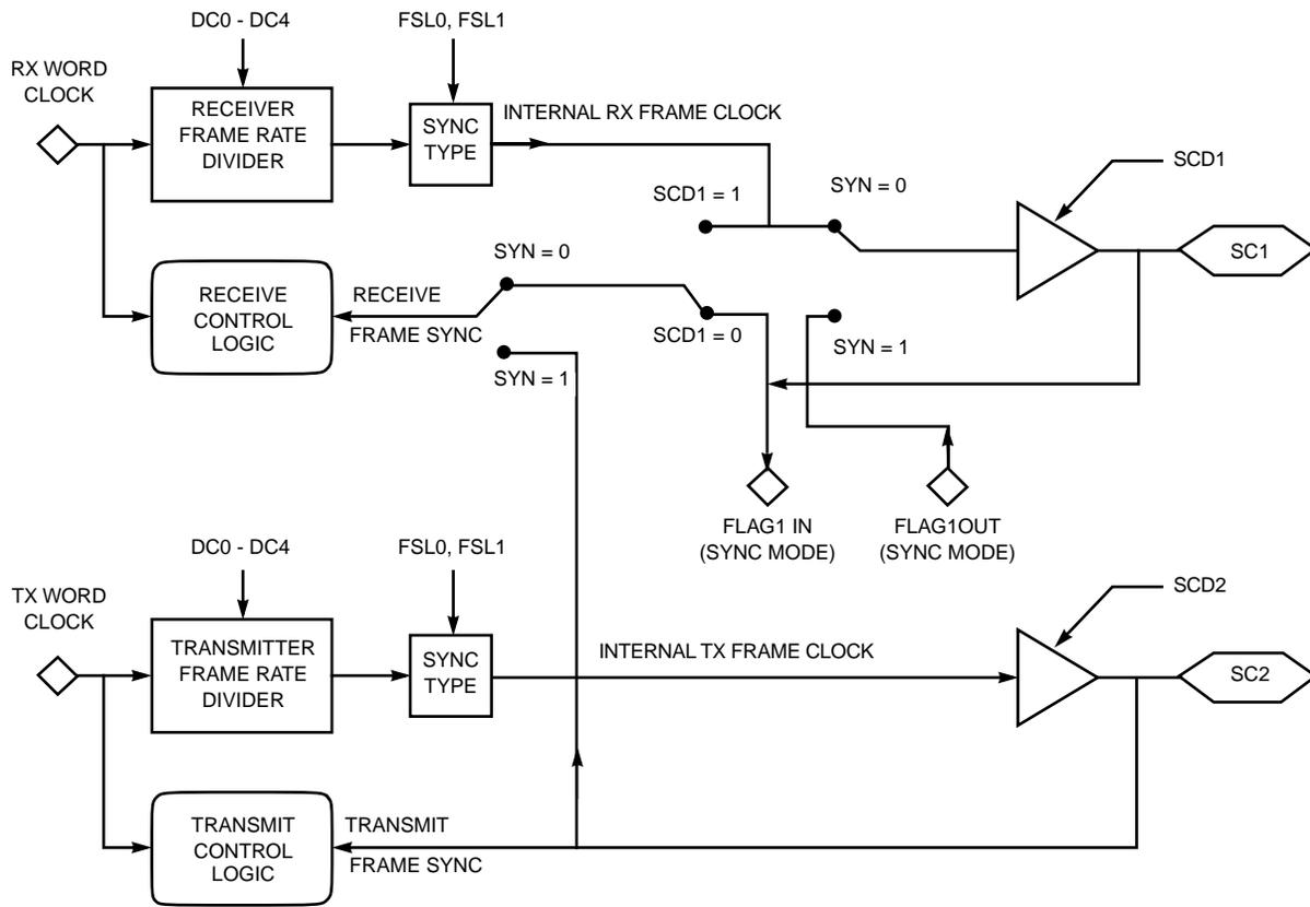
Figure 6-43 SSI Frame Sync Generator Functional Block Diagram
