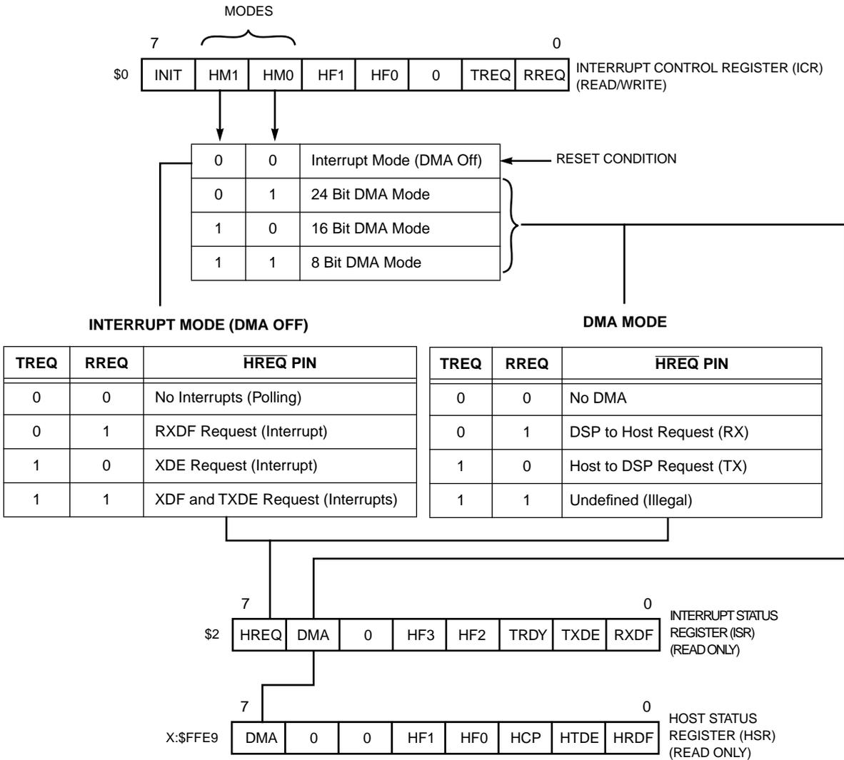
**Figure 5-38 Host Bits with TREQ and RREQ**
