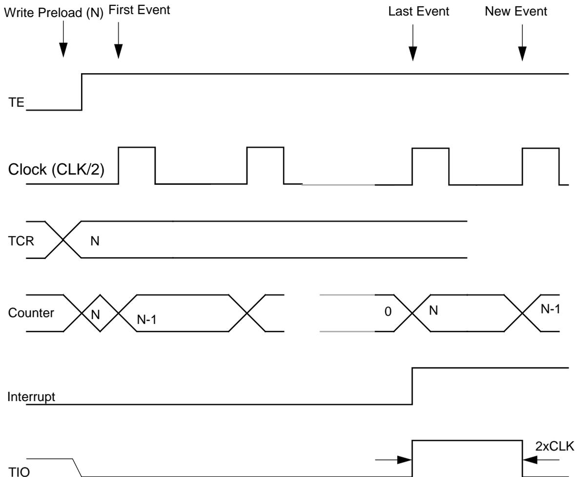
Figure 7-5 Standard Timer Mode, Internal Clock, Output Pulse Enabled (INV=0)
