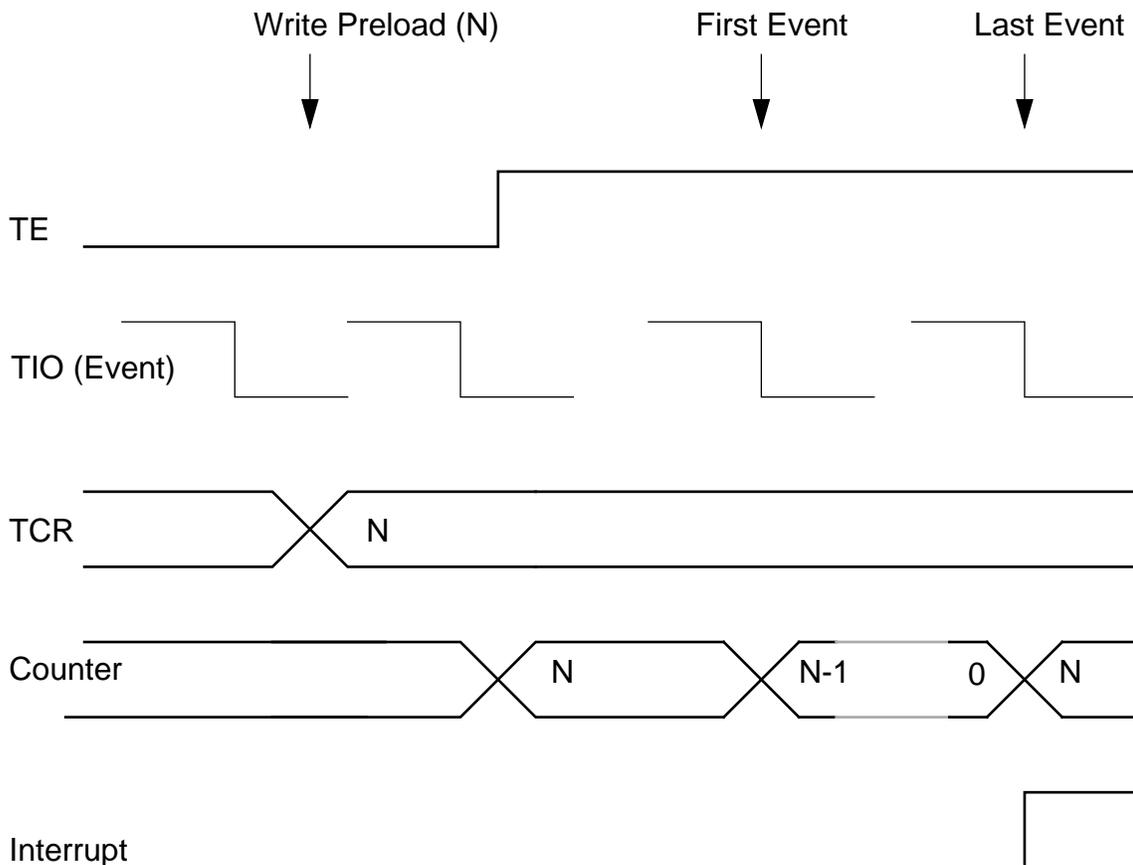
Figure 7-15 Standard Timer Mode, External Clock (INV=1)
