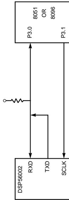
Figure 6-18 Synchronous Slave
