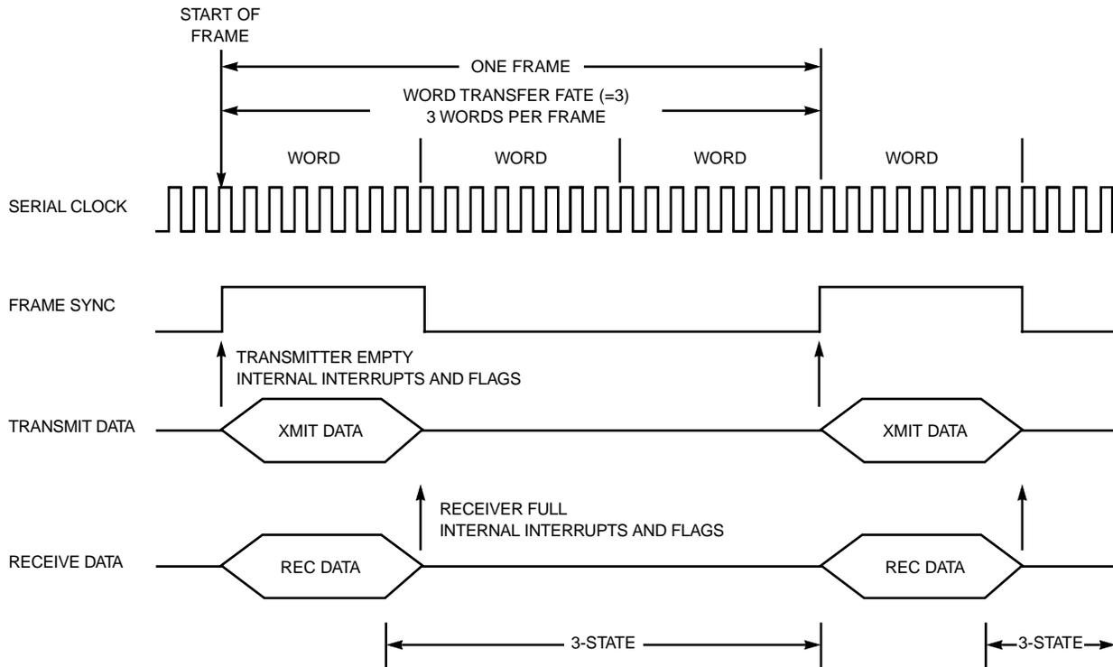
**Figure 6-62 Synchronous Communication**
