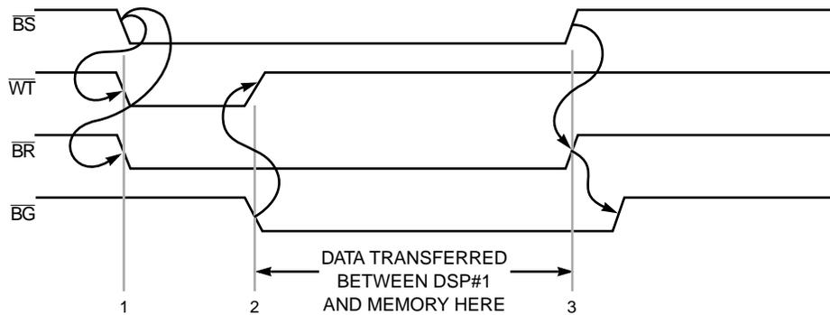
Figure 4-16 Two DSPs with External Bus Arbitration Timing
