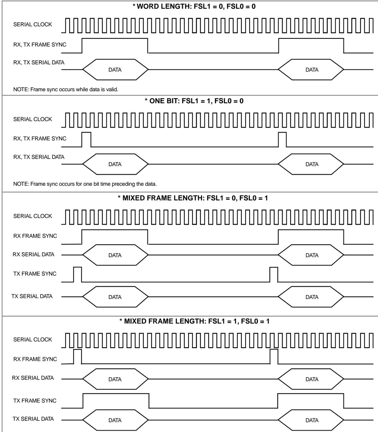
**Figure 6-68 CRB FSL0 and FSL1 Bit Operation**
